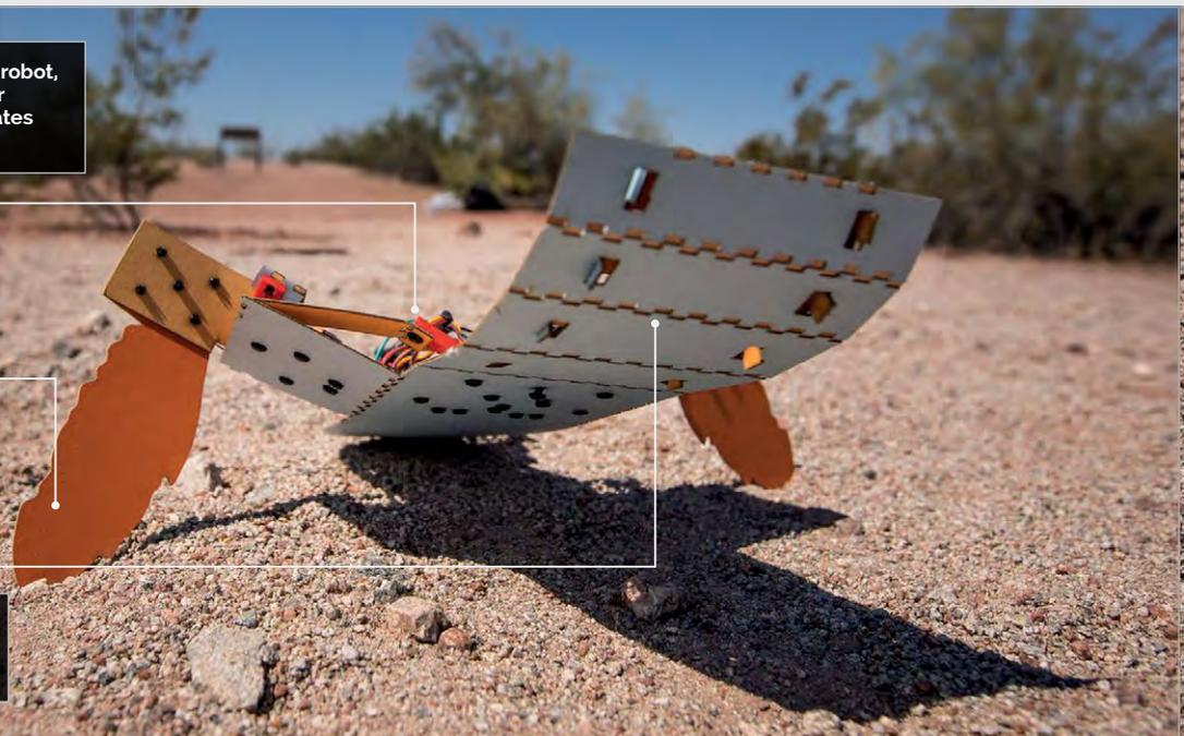
A Raspberry Pi Zero powers the robot, while a 16-channel, 12-bit motor driver from Adafruit communicates with the moving parts
