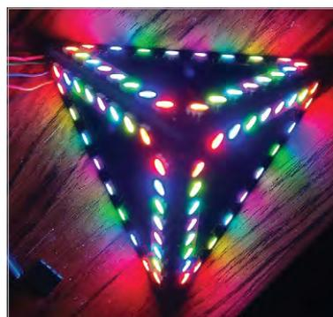
Indeed, that's what you'll be doing if you want to build a pyramid. After assembling the 3D shape from three triangles, held together using pieces of sticky tape, you'll need to solder bare wires between the input/output holes at each vertex, which is fairly fiddly.
