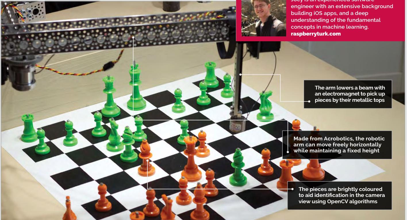
The arm lowers a beam with an electromagnet to pick up pieces by their metallic tops
