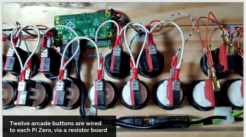
Twelve arcade buttons are wired to each Pi Zero, via a resistor board
